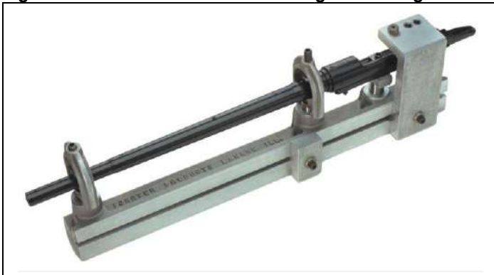
Figure 1. Mauser Barrel in Universal Sight Mounting Fixture
