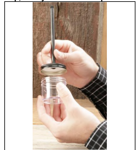
Fig. 1a. Drop Tube in Primer Catcher Cap, Ready to Attach to Cup
